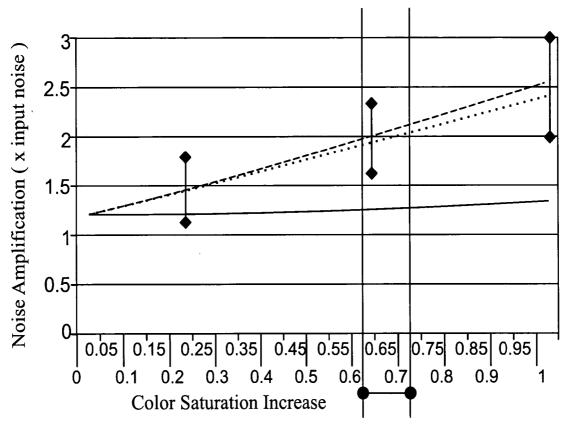
Just noticeable saturation difference (for CMOS imager at 200 Lux luminance)
